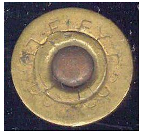
Adams MK1 .450 (separate iron base disk) 1868 - MK2 (separate brass base disk) 1877
