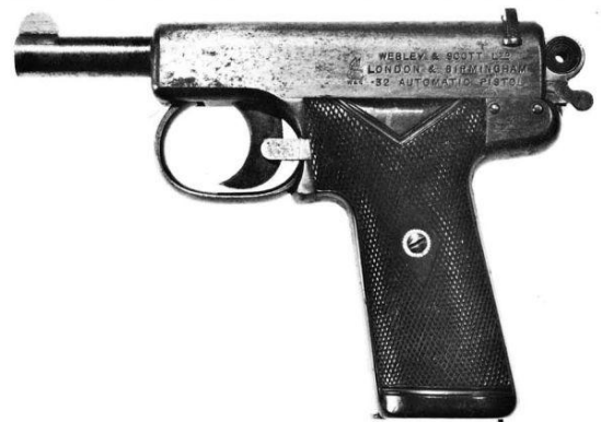
Webley & Scott semi automatic pistol, cal.32, model of 1905. Very early model with safety lever located next to the hammer. ( www.worldguns.ru )
