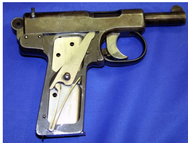
Webley & Scott Semi Auto Pistol .32 Cal sn 103056 with right side grip removed to show unique "V" spring
